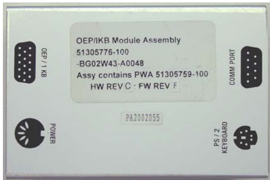
Figure 2-6 OEP/IKB Module Assembly (51305776-100) Top View.
