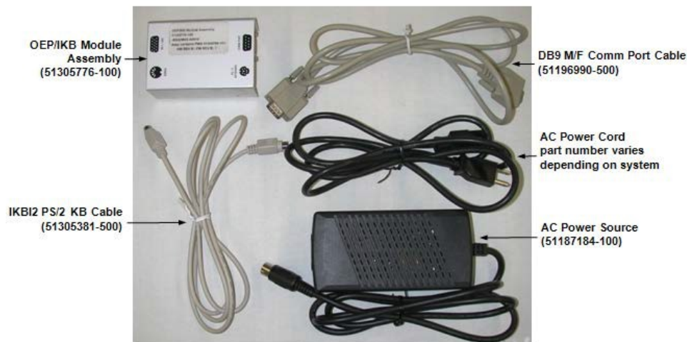
Figure 2-1 Honeywell OEP/IKB Adapter Kit Components
