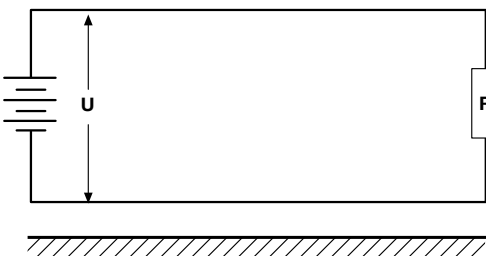
Figure 9 Network insulated from earth
