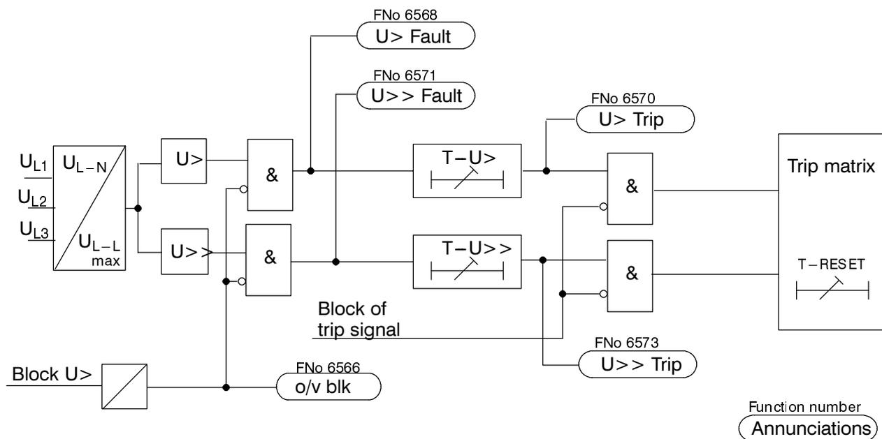
Figure 4.6 Logic diagram of the two-stage overvoltage protection
