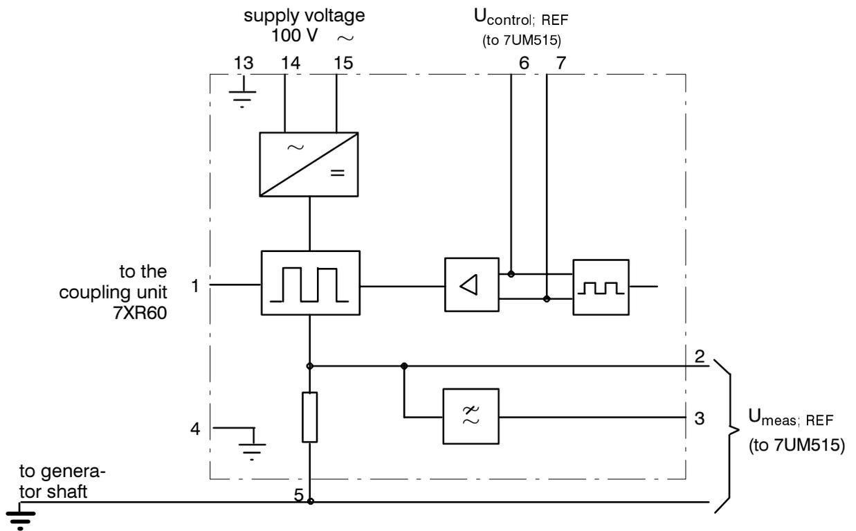
Figure 2.7 Schematic diagram of controller unit, type 7XT7000-0B
