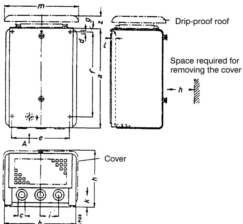
3PP1 with degree of protection IP 20 (IP 23 with drip-proof roof)
