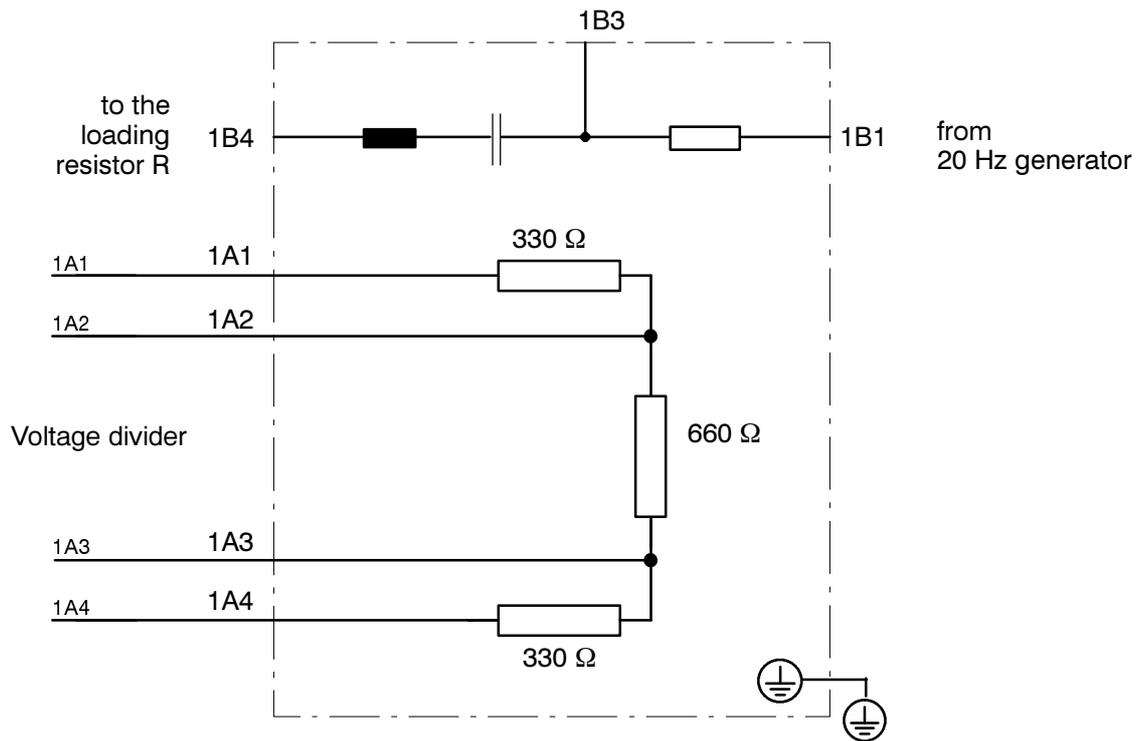
Figure 2.6 Schematic diagram of 20 Hz band-pass filter, type 7XT3400-0\*A00
