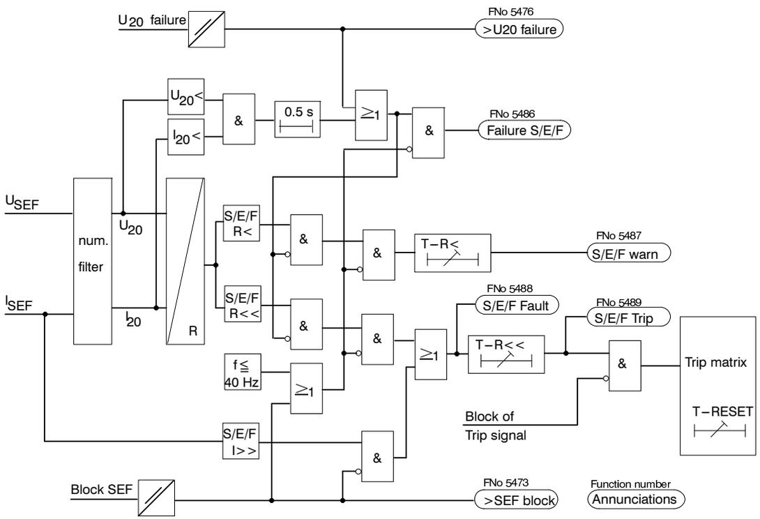
Figure 4.9 Logic diagram of the stator earth fault 100% protection
