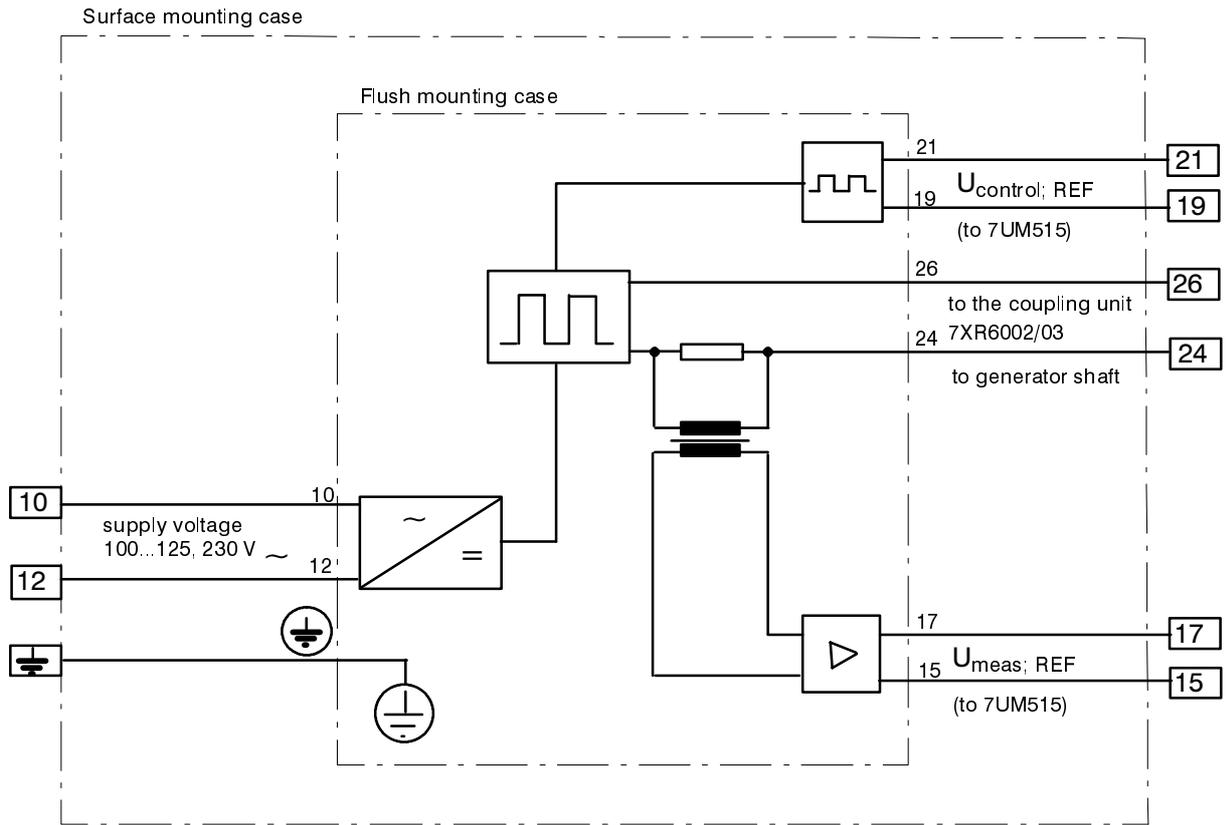
Figure 2.8 Schematic diagram of controller unit 7XT7100-0\*A00
