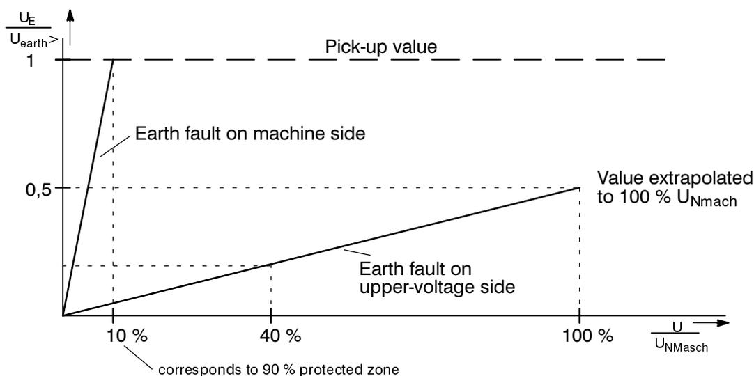
Figure 6.11 Neutral displacement voltage during earth faults
