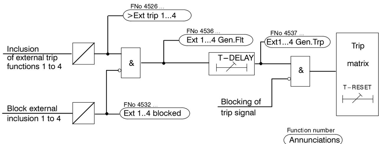
Figure 4.18 Logic diagram of one external trip command channel
