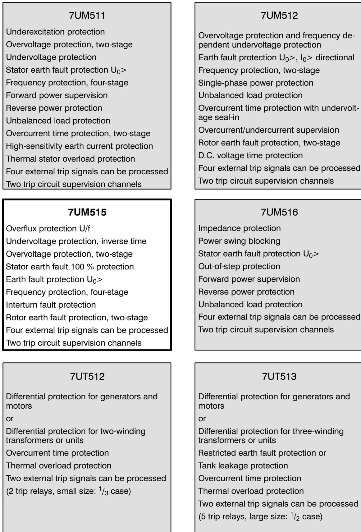
Figure 1.1 Survey of the numerical machine protection series
