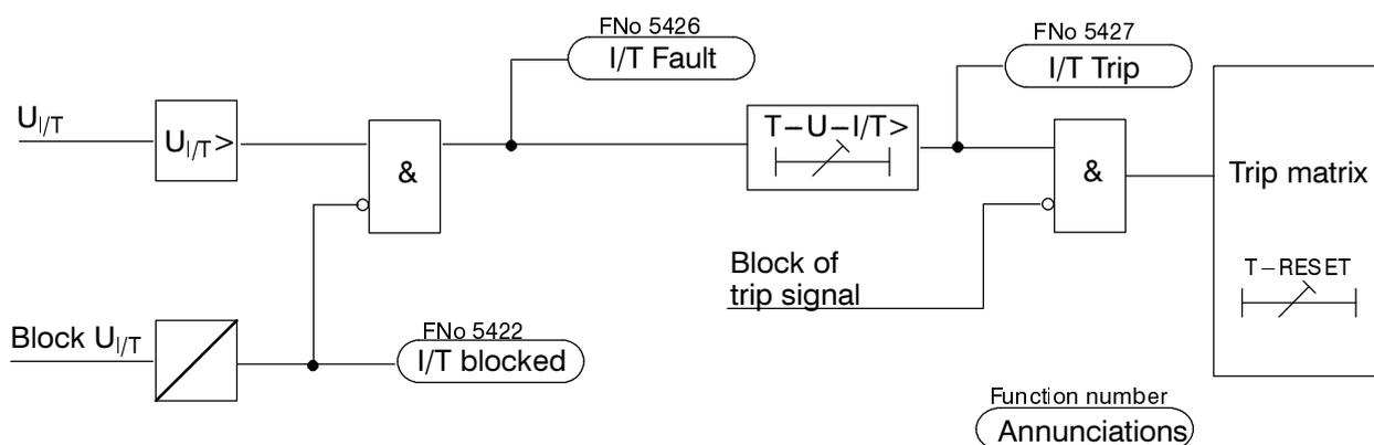
Figure 4.13 Logic diagram of the interturn fault protection
