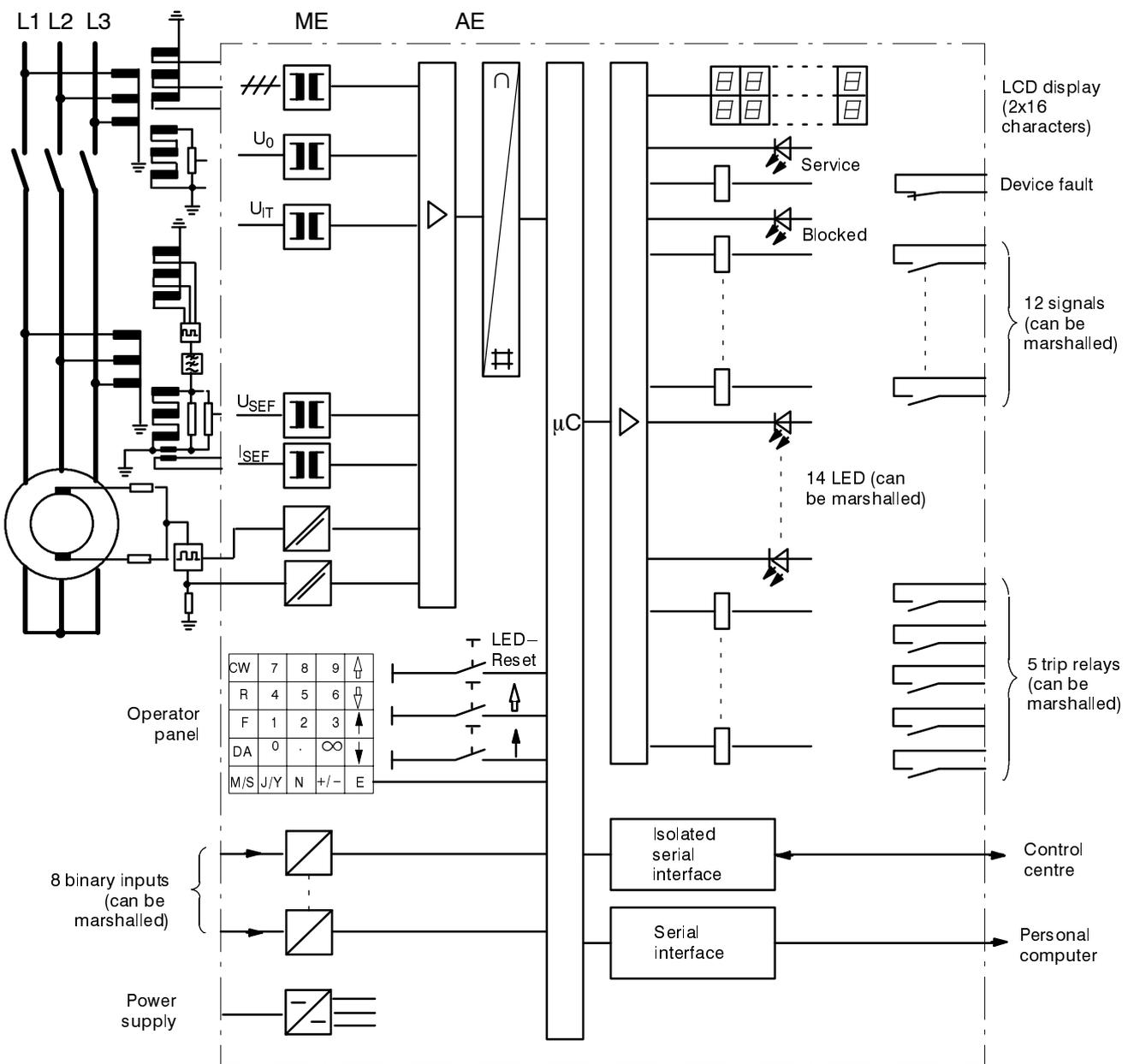
Figure 4.1 Hardware-structure of machine protection relay 7UM515
