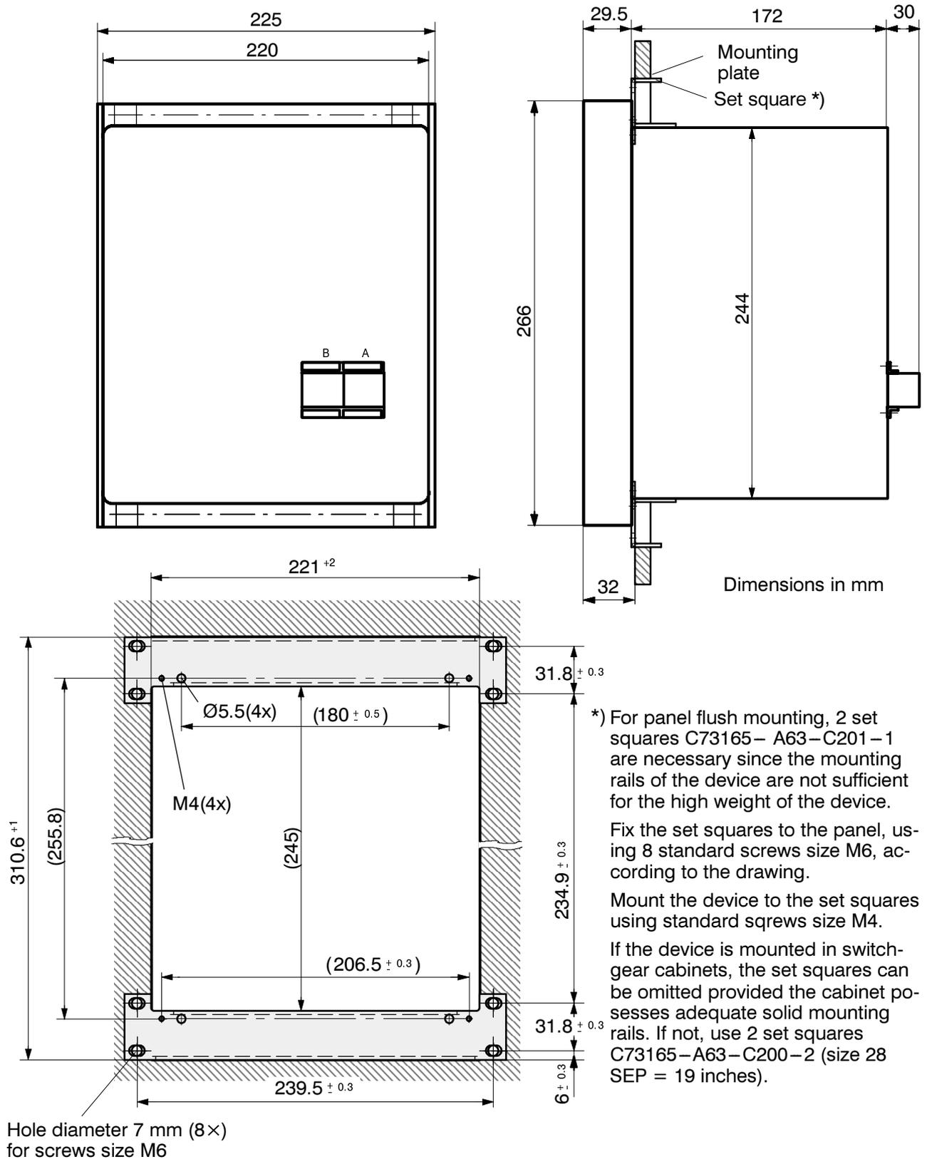
Figure 2.12 Dimensions of 20 Hz band-pass filter, type 7XT3400–0\*A00 for panel flush mounting or cubicle installation
