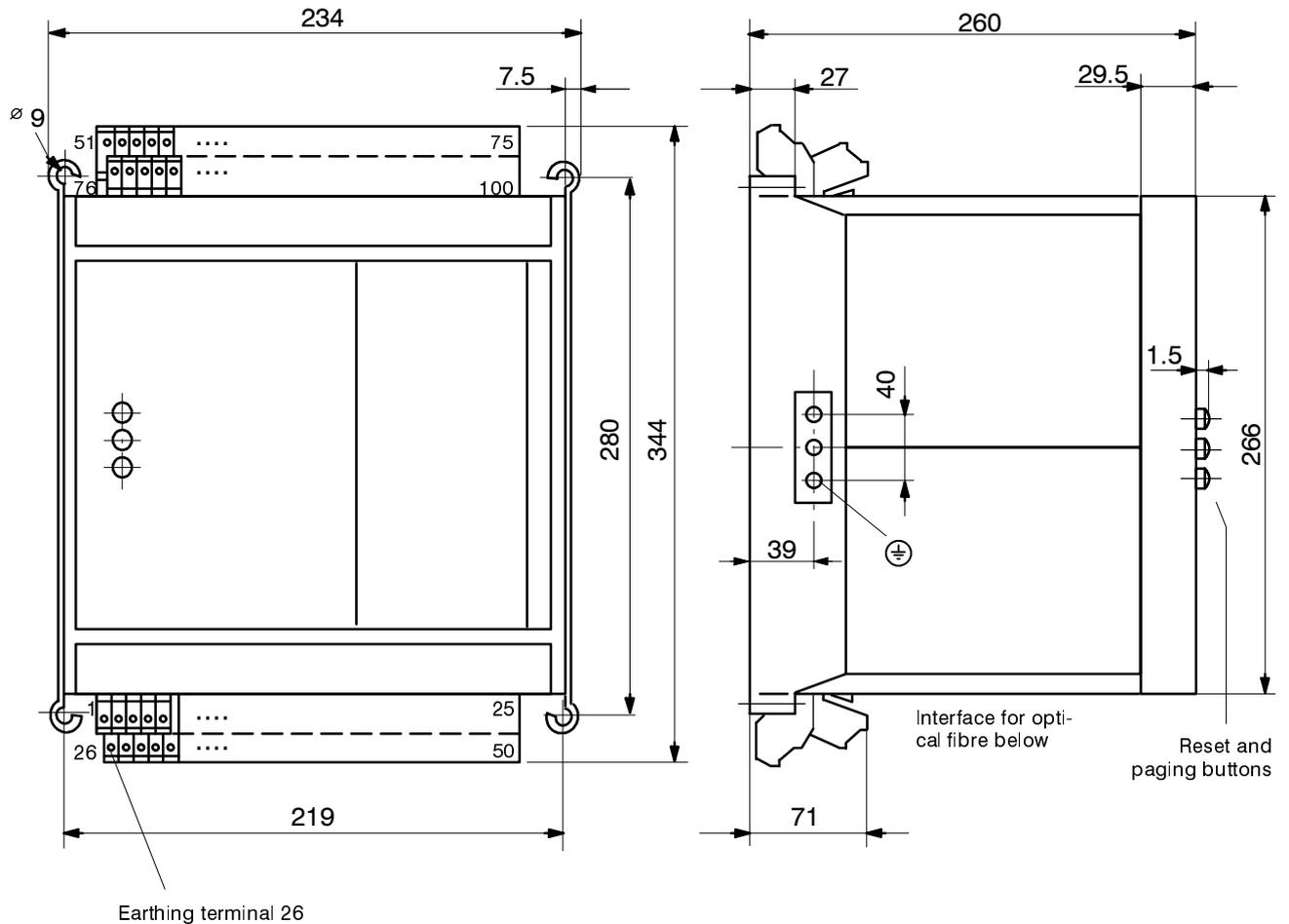
Max. 100 terminals for cross-section max. 5 mm<sup>2</sup>
