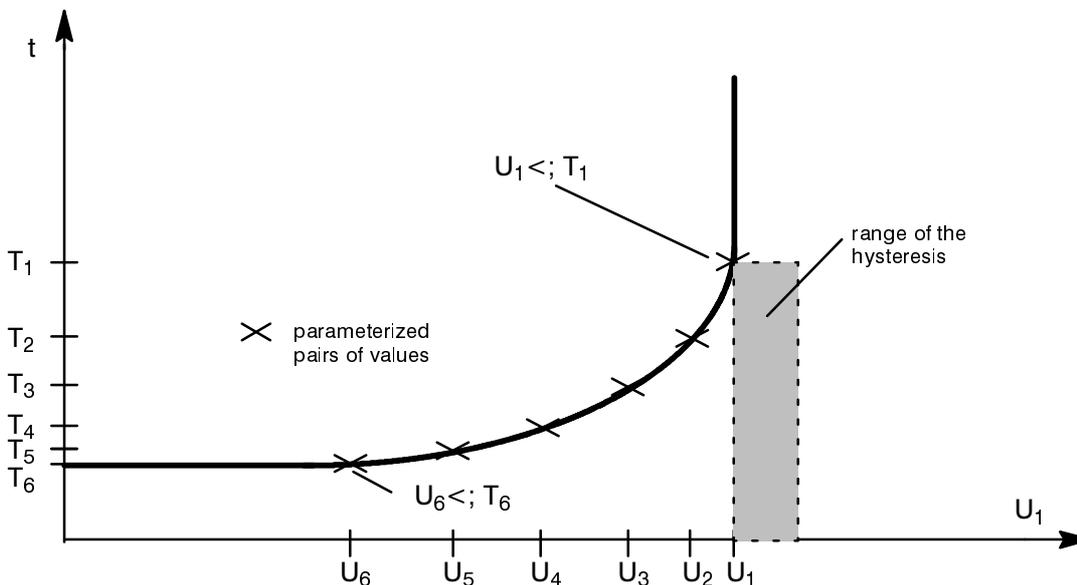
Figure 4.4 Tripping time characteristic of undervoltage protection – example
