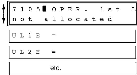
Message to be displayed in the **1st** display line during operation. Any of the operational measured values according to Section 6.4.4 can be selected as messages in the quiescent state of the relay by repeatedly depressing the “No”–key **N**; The value selected by the entry key **E** under address 7105 will appear in the **first** line of the display.
