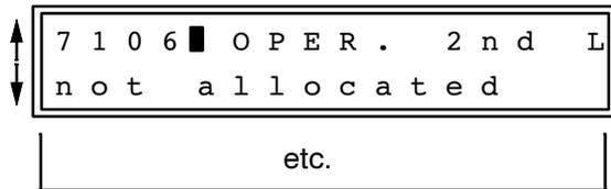
Message to be displayed in the **2nd** display line during operation. The value selected by the entry key **E** under address 7106 will appear in the **second** line of the display.
