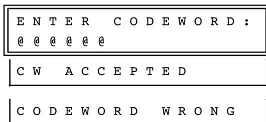
The entered characters do not appear in the display, instead only a symbol @ appears. After confirmation of the correct input with **E** the display responds with **CW ACCEPTED**. Press the entry key **E** again.
