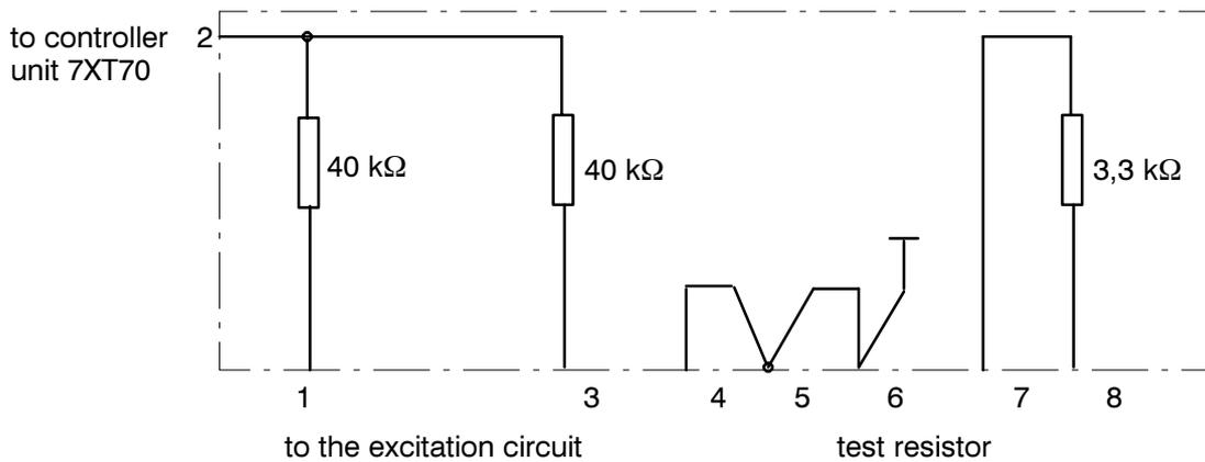
Figure 2.9 Schematic diagram of coupling unit, type 7XR6002 and 7XR6003
