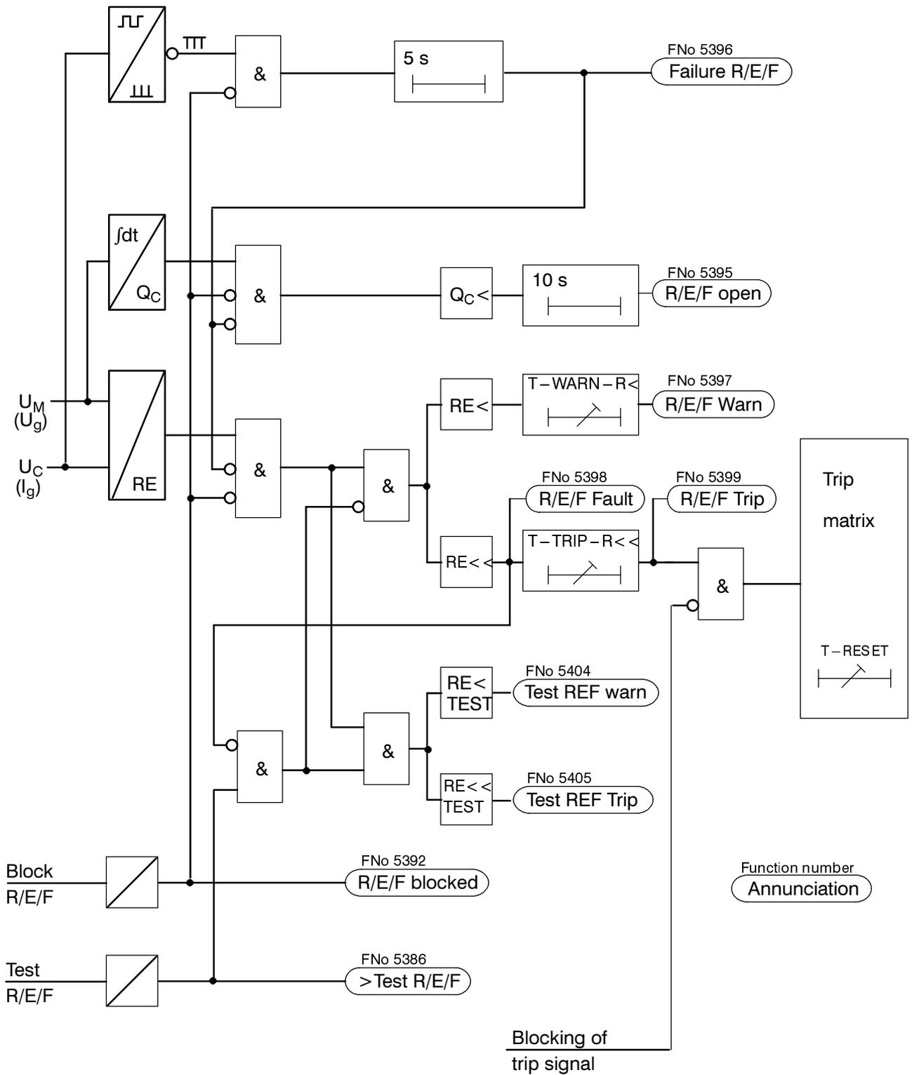
Figure 4.16 Logic diagram of the rotor earth fault protection
