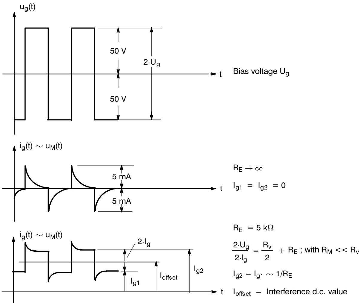
Figure 4.15 Time diagram of measured values, examples for measured value formation
