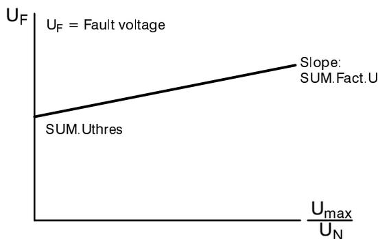
Figure 4.21 Voltage sum monitoring (voltage plausibility check)
