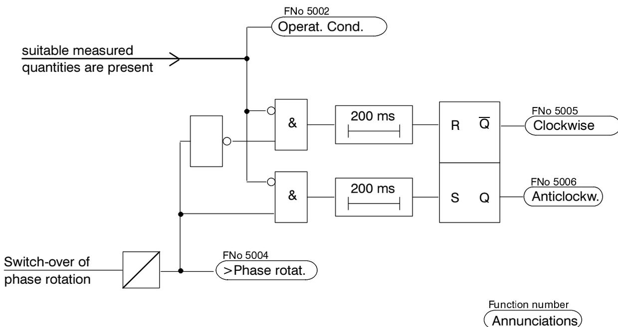
Figure 4.19 Logic diagram of the switch-over of the phase rotation
