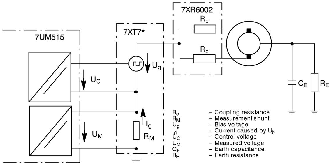
Figure 4.14 Connection scheme of rotor earth fault protection
