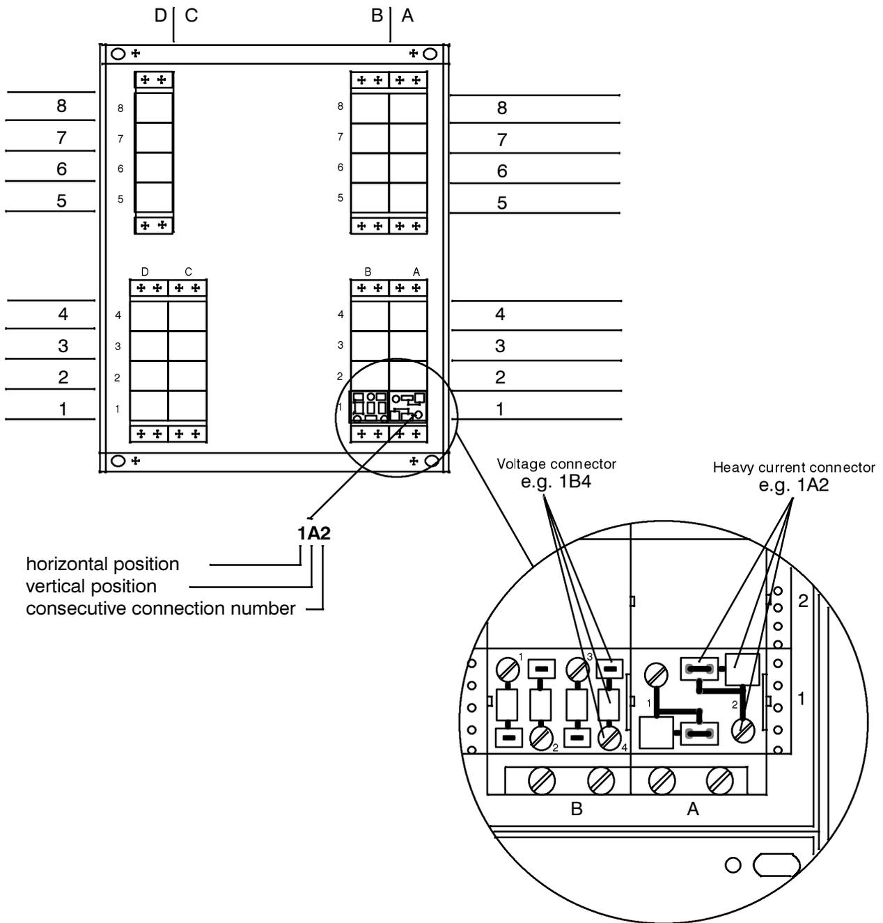
Figure 2.1 Connection plugs (rear view) – housing for flush mounting – example
