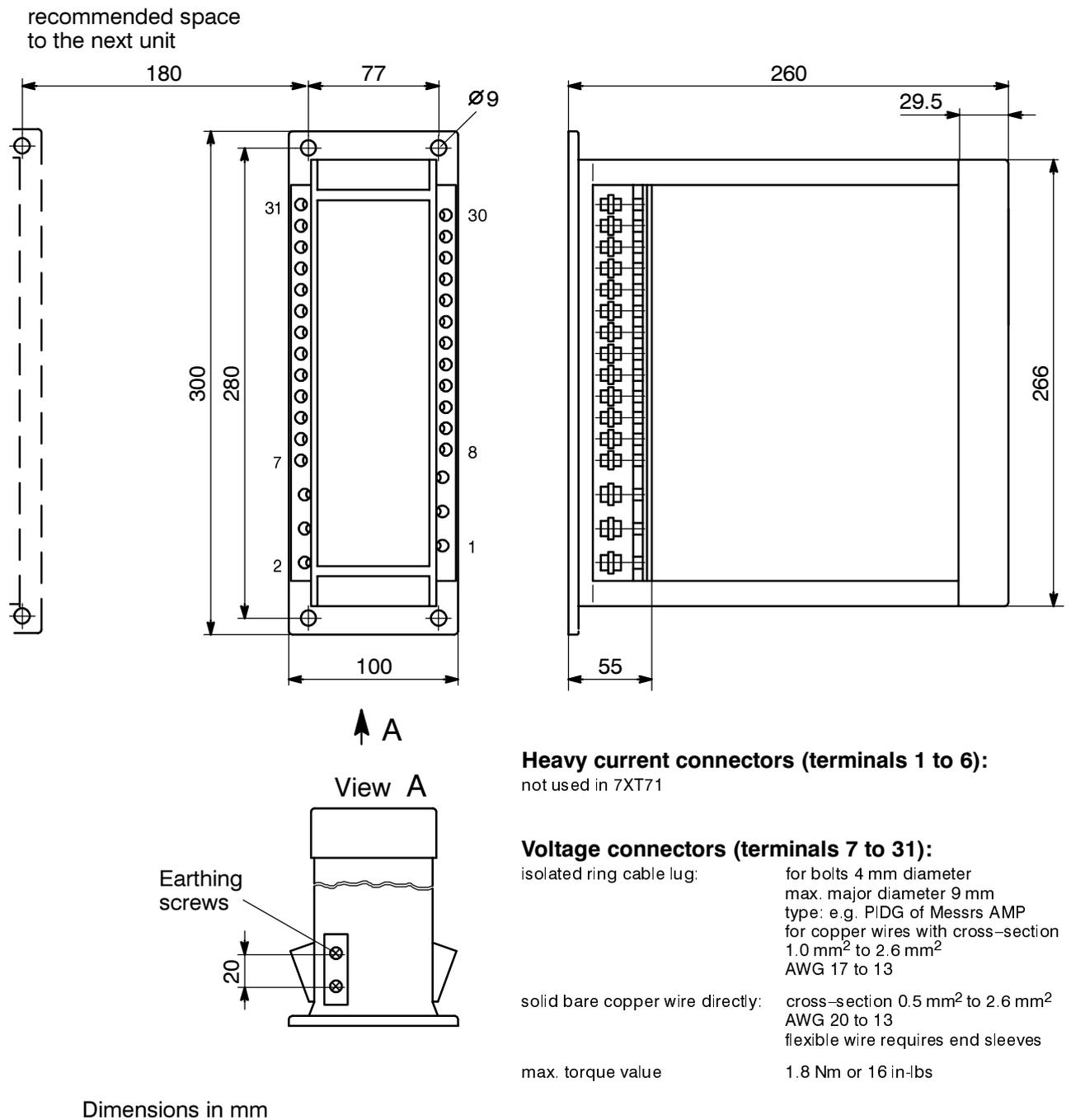
Figure 2.15 Dimensions of controller unit, type 7XT7100-0BA00 for panel surface mounting with terminals at both sides
