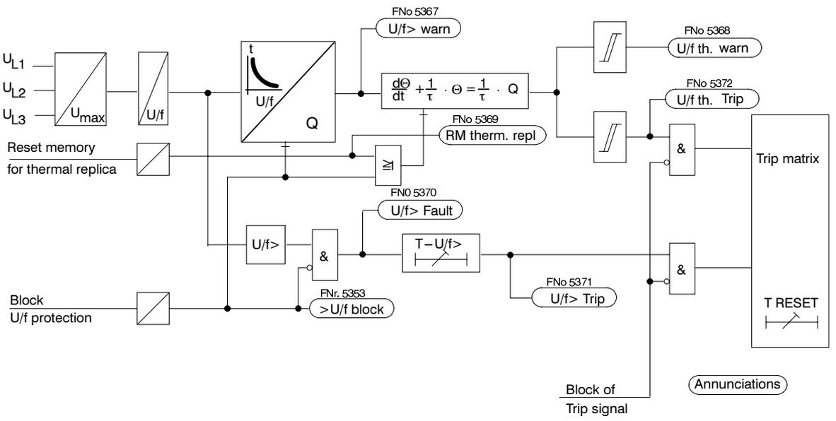
Figure 4.3 Logic diagram of the overflux protection
