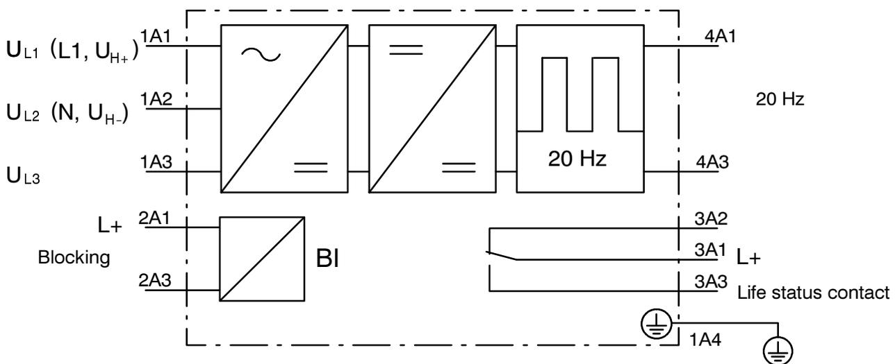
Figure 2.5 Schematic diagram of 20 Hz generator, type 7XT3300-0\*A00
