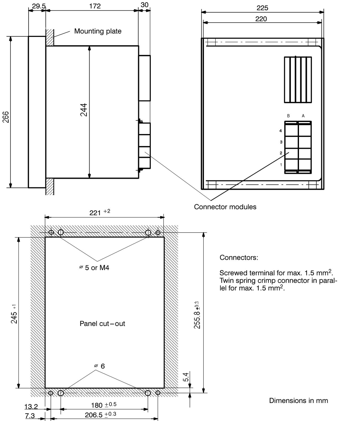
Figure 2.11 Dimensions of 20 Hz generator, type 7XT3300-0\*A00 for panel flush mounting or cubicle installation
