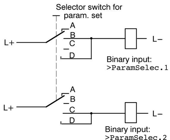
Figure 6.3 Connection scheme for parameter change-over via two binary inputs
