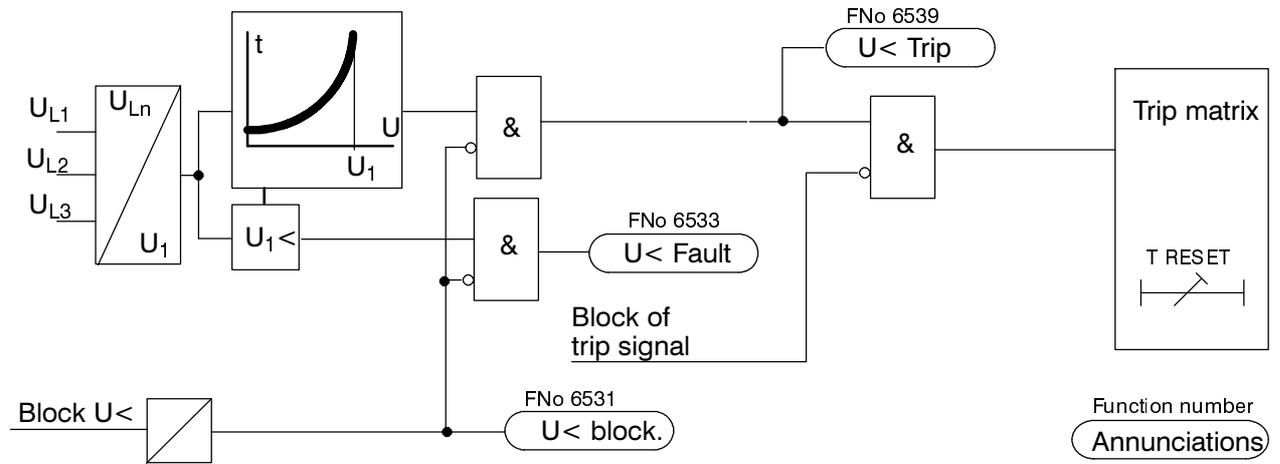
Figure 4.5 Logic diagram of undervoltage protection
