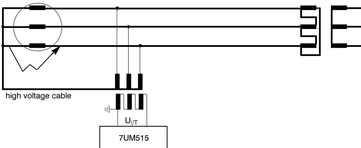
Figure 4.12 Connection scheme of interturn fault protection
