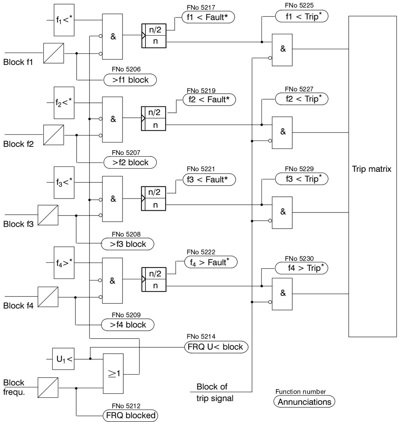
\* The pick-up symbols and the annunciations are illustrated for the preset configuration of the frequency protection. If the configuration is changed, the symbols < and > may appear interchanged.
