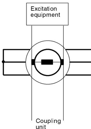
Figure 6.7 Excitation equipment fed via slip rings
