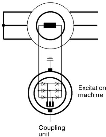
Figure 6.6 Excitation via rotating rectifiers with measurement brushes
