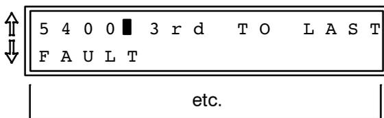
Beginning of the block "Fault annunciations of the third to last fault"
