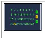
Outputs 1 – 16 Power Present Outputs 17 – 32 Power Present Terminal Block Present 32 green/yellow LEDs on the module indicate the ON/OFF status of points 1 through 32. These LEDs are green when the corresponding outputs are on, and yellow if the outputs are faulted. They are off when the corresponding outputs are off.
