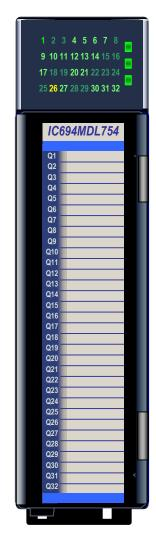
The **12/24 volt DC, ESCP 0.75A Positive Logic Output** module, IC694MDL754, provides 32 discrete outputs in two isolated groups of 16. Each group has its own common. The outputs are positive logic or sourcing type outputs; they switch the loads on the positive side of the power supply, and supply current to the load. The outputs can switch user loads over the range of +12 to +24 VDC (+20%, -15%) and can source a maximum current of 0.75 Amps per point.
