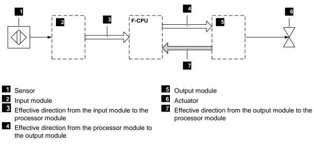
Figure 32: Effective Direction Associated with Noise Blanking and Output Noise Blanking
