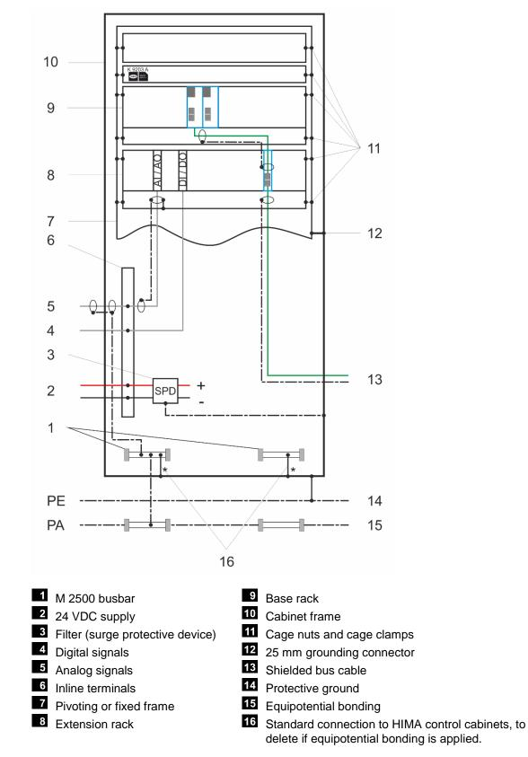
Figure 35: Grounding and Shielding Concept of the HIMA Standard Cabinet
