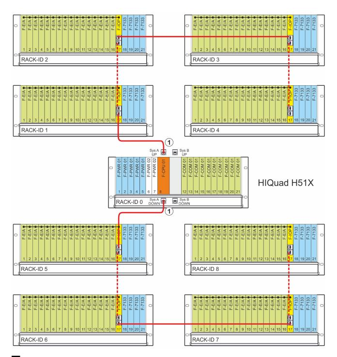
1 System bus interfaces on the rear side of the base rack
