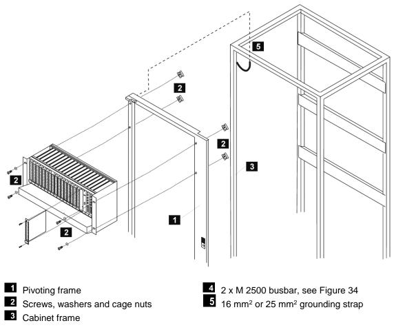
Figure 33: Grounding Connectors for Racks
