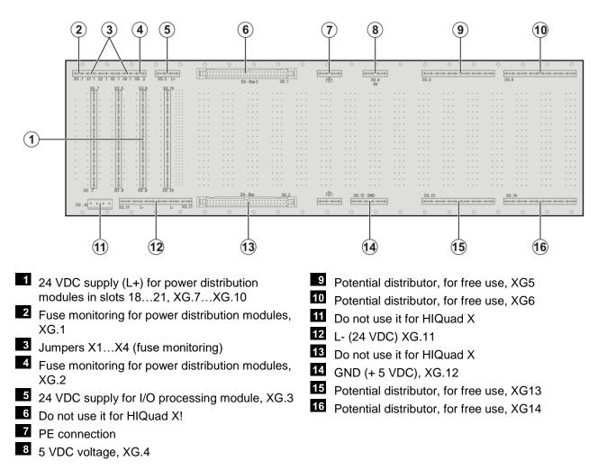
Figure 18: Rear View of Extension Rack Backplane
