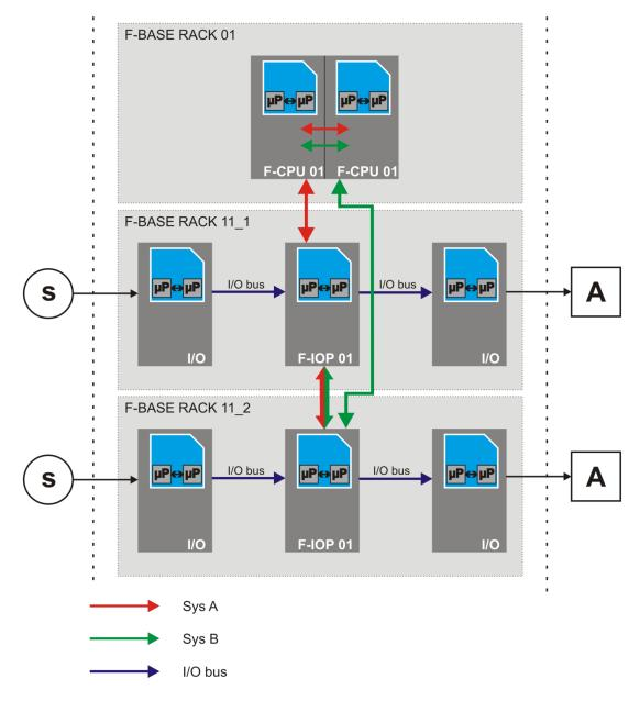
Figure 4: Example of Safe H51X Redundant Operation (1002)
