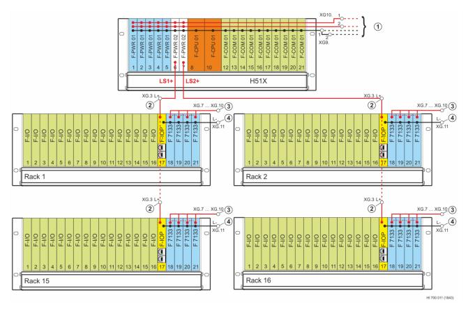
Connection to redundant power supply units, see Figure 20
