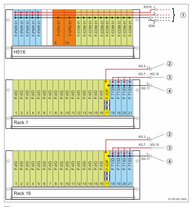
Connection to redundant power supply units, see Figure 20
