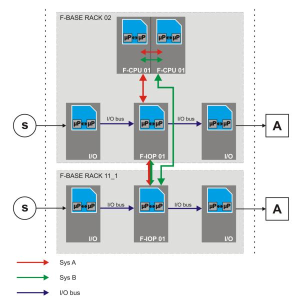
Figure 9: Example of Safe H41X Redundant Operation (1002)
