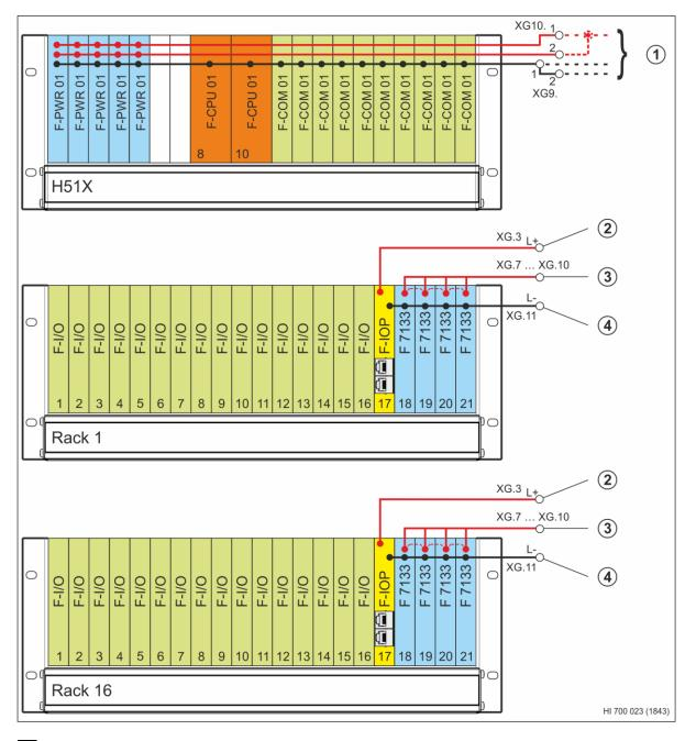
Connection to one or redundant power supply units, see Figure 19
