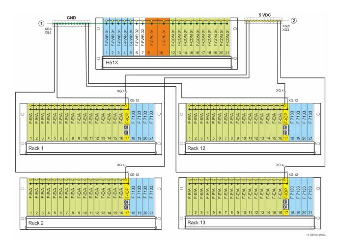
GND connectors (XG4 and XG5) on the rack rear side
