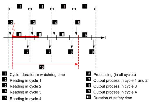
Figure 30: Transient Interference
