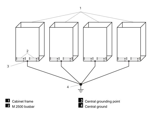
Figure 36: Control Cabinets with Central Ground
