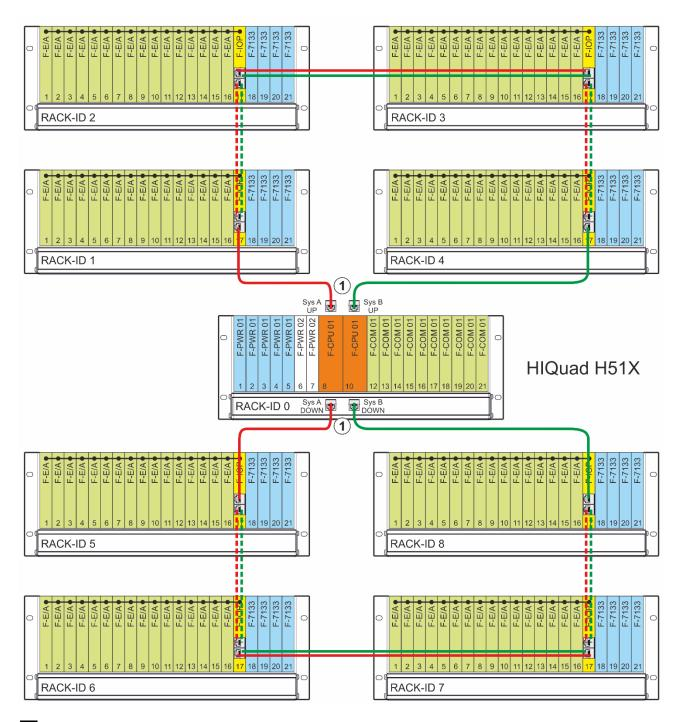
System bus interfaces on the rear side of the base rack
