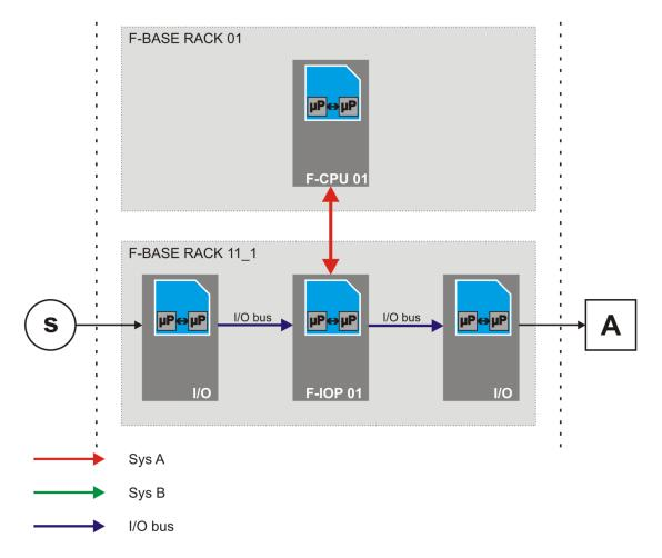
Figure 2: Example of Safe H51X Mono Operation (1002)
