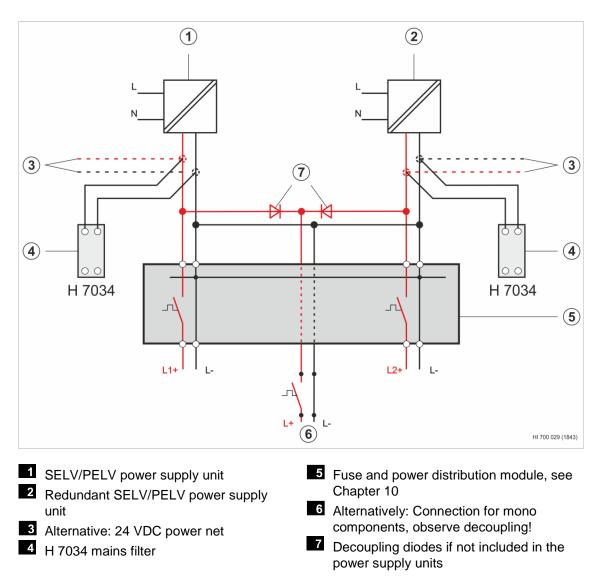
Figure 20: Redundant 24 V Power Supply
