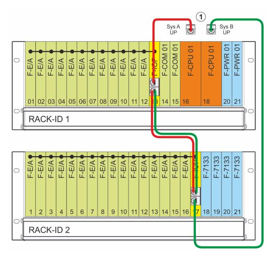
System bus interfaces on the rear side of the base rack
