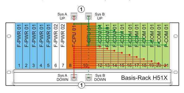
System bus interfaces on the rear side of the base rack
