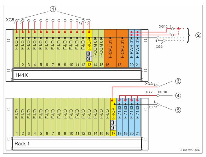
Inline terminals XG5.1...XG5.13 to 24 V power supply, XG5.13 for connecting to the I/O processing modules.
