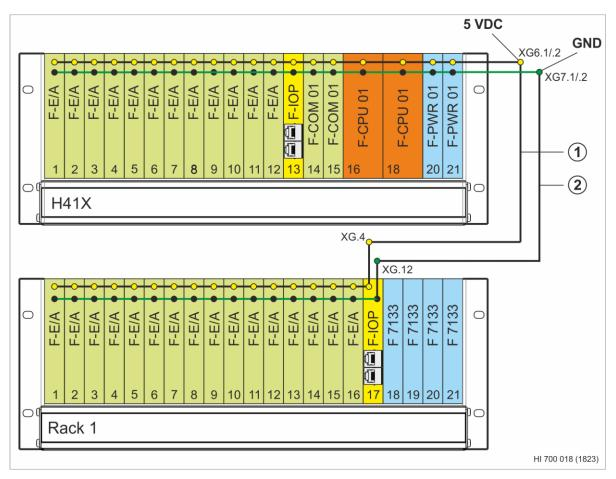
1 5 VDC connector XG6.1.2 (base rack), XG.4 (extension rack).
